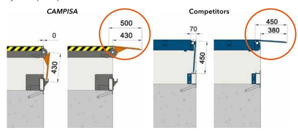
The **Swing lip** dock levellers are more economic, the vehicle docks to the loading bay and contacts the bumper, the leveller is raised, the lip is opened and laid onto the truck bed, and loading procedure starts.
