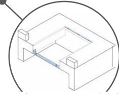
**FLY**: application on suspended dock leveller. The self-bearing front beam can be easily installed in case of tail lift clearance.
