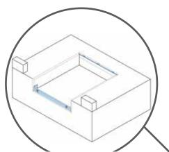
**STAR**: application on pit built in traditional way. Front beam fixing by expansion bolts and rear hinges
