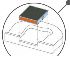
**CAST**: application on finished leveller with frame. To be levelled at final pavement and cast.
